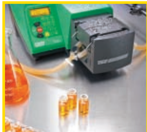
High accuracy batch filling of 10ml bottles
